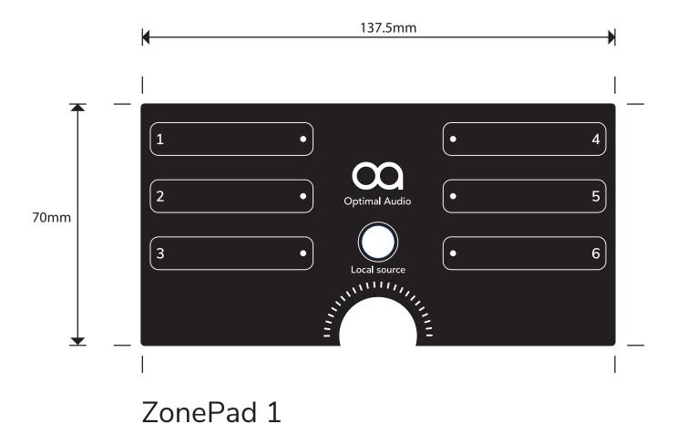
This template is setup for 1 colour print and is shown at 1:1 scale to be inserted into a ZonePad 1 face panel. Please ensure that printing output is at 100%, with dimensions of 137.5mm width and 70mm height. Suitable for printing on an A4 desktop printer or use as a template for commercial printing. A guideline template for die-cutting is on Page 2 of this document.
